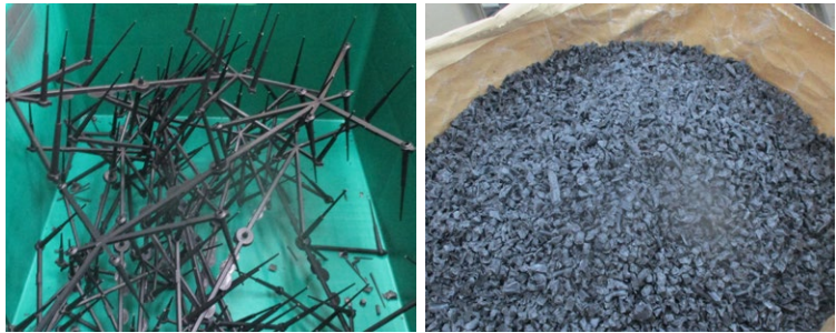
Resin waste from the mold injection process pulverized for use as recycled material
