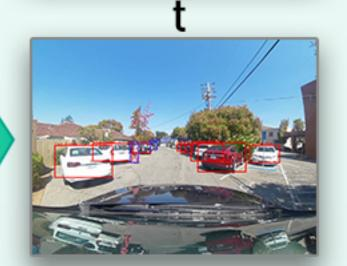
Temporal propagation of convolutional neural network detection with no latency
